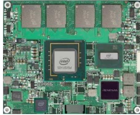
Figure 4. Radisys Procelerant Z500 85mm x 70mm Board Compatible with Type 2 COM Express Pinout
