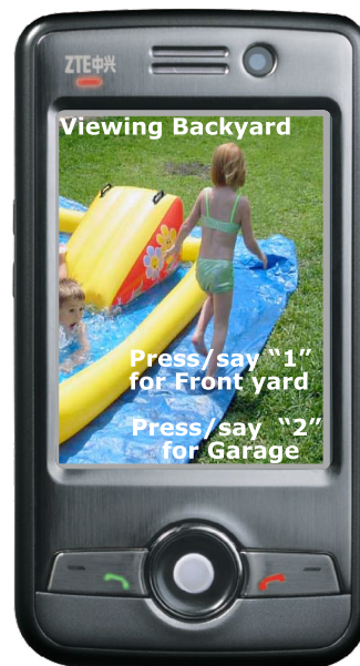
Example Mobile Surveillance Application using IVVR, Text Overlay, and Automatic Speech Recognition (ASR)
