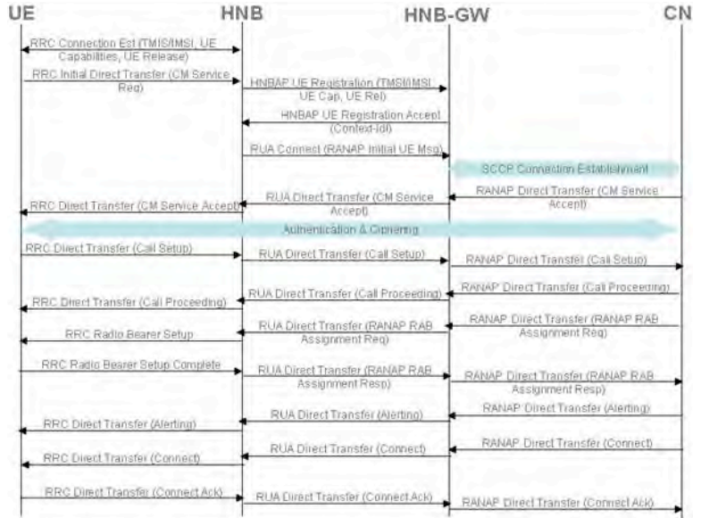
Figure 9. End-to-End Signaling for Mobile-Originated Voice Call
