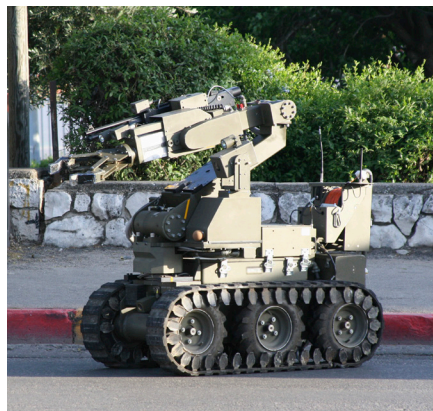
Figure 1. Talon unmanned ground vehicles made by Foster-Miller are rugged, lightweight tracked vehicles widely used for explosive ordnance disposal, reconnaissance, communications, sensing, security, defense and rescue.
